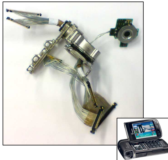
Micro-coaxial Cable Harness in a Hinged Mobile Phone
